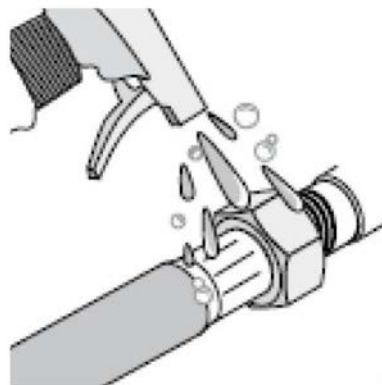
Test all connections for gas leaks using a soapy solution.
